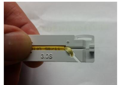
3. Lay the cable into the cleaving fixture. Twirl the kevlar strand and insert into the hole as shown.
